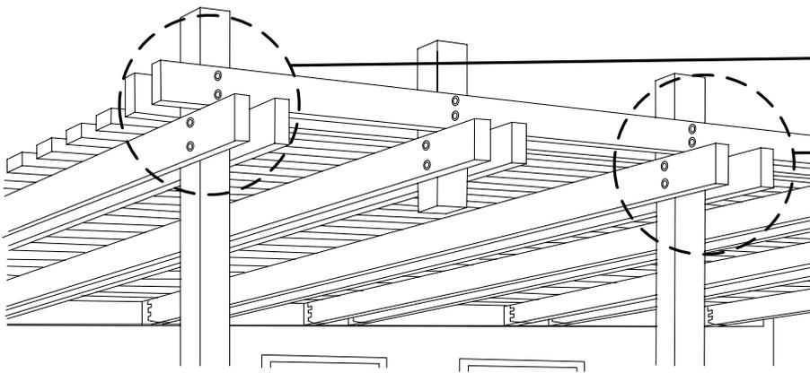
TWO 1/2" DIA. THRU-BOLTS (W/ WASHERS), PER CONNECTION AS SHOWN
