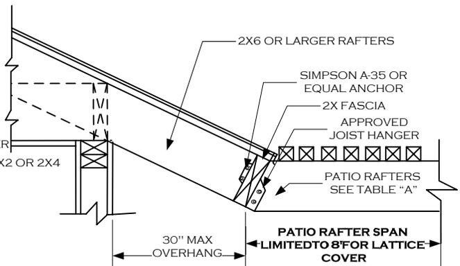
**NOTE:** VERIFY STRUCTURAL SOUNDNESS OF ROOF RAFTERS FOR DECAY OR TERMITE DAMAGE, AND REPLACE WITH LIKE MATERIALS AS NEEDED, AFTER CONSULTATION WITH THE BUILDING DEPARTMENT.
