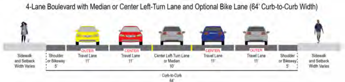
Figure 3-5 Planned 4-Lane Boulevard Typical Section
