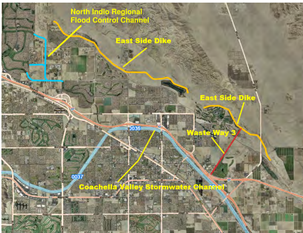
Figure 2-3 City of Indio Regional Drainage Facilities -CVWD
