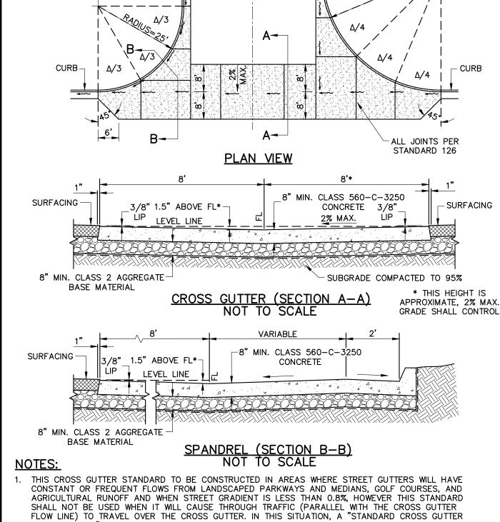
AGRICULTURAL RUNOFF AND WHEN STREET GRADIENT IS LESS THAN 0.8%, HOWEVER THIS STANDARD SHALL NOT BE USED WHEN IT WILL CAUSE THROUGH TRAFFIC (PARALLEL WITH THE CROSS GUTTER FLOW LINE) TO TRAVEL OVER THE CROSS GUTTER. IN THIS SITUATION, A "STANDARD CROSS GUTTER AND SPANDREL" PER STANDARD 137 SHALL BE USED.
