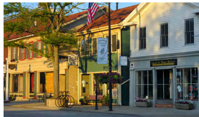
To ensure that an environment is interesting to walk through, commercial ground floors shall have frequent doors and clear and ample fenestration.
